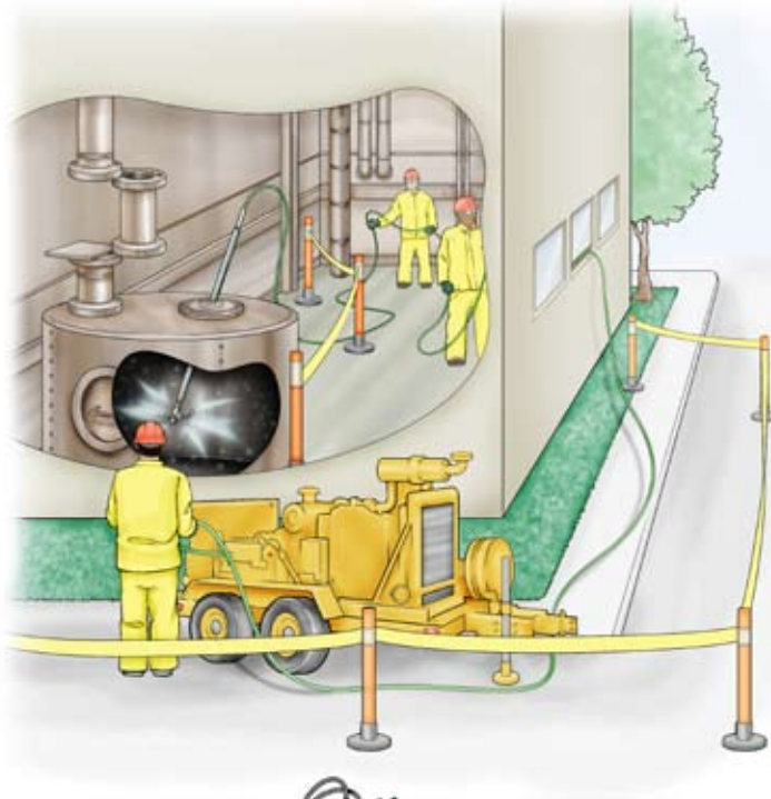
Figure 11b. Mechanized shell-side bundle cleaning using a remotely operated boom.
